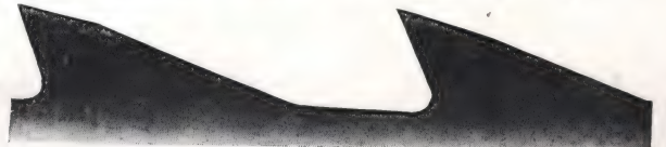
Shape O. Space 1\frac{1}{2} " to 2\frac{1}{2} ". Depth \frac{3}{8} " to \frac{7}{8} ".
